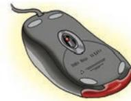
**Fig 1.12** Optical mouse (as seen from below)
